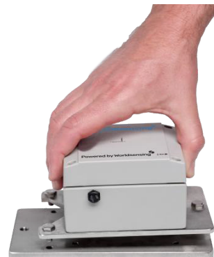
Fig. 6: The Tilt90-i mounted on a double plate for horizontal surface mounting (LS-ACC-IN15DP). This is suitable for applications that need avoid opening the casing during installation. The plate includes a threaded hole available for installing a monitoring prism or a button head screw for precise leveling.
