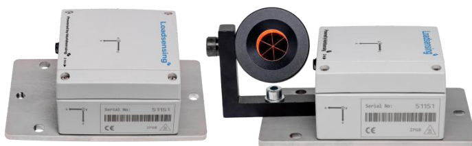
Fig. 3: Versatile horizontal surface mounting plate (LS-ACC-IN15-HP), recommended for both horizontal and vertical mounting. The plate has three clearance holes for MB anchor rods and an MB threaded hole available for installing a monitoring prism or a button head screw for precise leveling.
